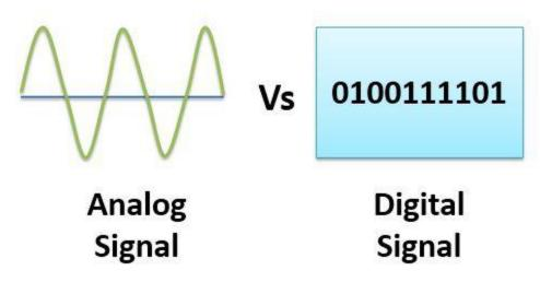
Analog and Digital are the different forms of signals. Signals are used to carry information from one device to another. Analog signal is a continuous wave that keeps on changing over a time period. Digital signal is discrete in nature.
