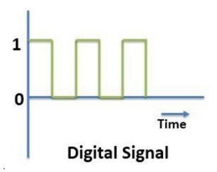
Digital signal can be further decomposed into simple sine waves that are called harmonics. Each simple wave has different amplitude, frequency and phase. Digital signal is described with bit rate and bit interval. Bit interval describes the time require for sending a single bit. On the other hand, bit rate describes the frequency of bit interval.
