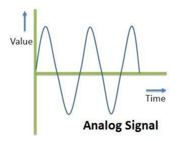
An analog signal is not immune to noise hence, it faces distortion and decrease the quality of transmission. The range of value in an analog signal is not fixed.
